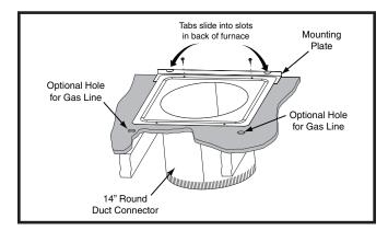
Figure 15. Round Duct Connector
