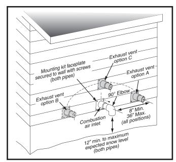
Figure 1. Inlet & Exhaust Pipe Clearances
