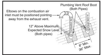
**Figure 4. Vertical Vent Termination**
