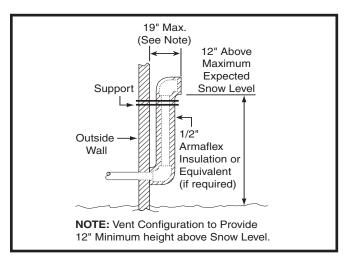
Figure 3. Alternate Horizontal Vent Installation
