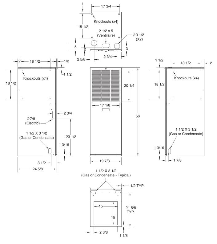
Figure 24. Front Return Cabinets (Without Coil Box)
