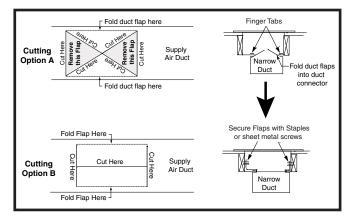
Figure 12. Screw-Down Duct Connector
