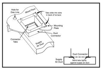
Figure 11. Finger Tabbed Duct Connector
