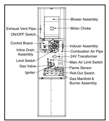
Figure 23. Furnace Components
