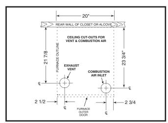
Figure 10. Ceiling Cut-Out Dimensions
