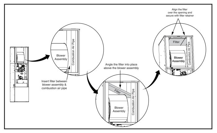
Figure 7. Filter Installation
