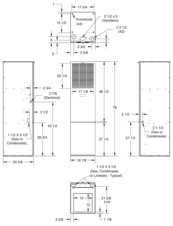
Figure 25. Front Return Cabinets (With Coil Box)
