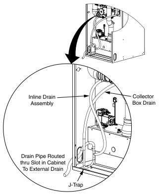
Figure 17. Condensate Drainage
