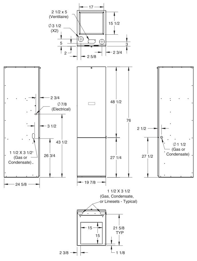
Figure 27. Top Return Cabinets (With Coil Box)
