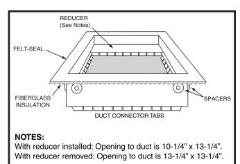
Figure 8. Duct Connector
