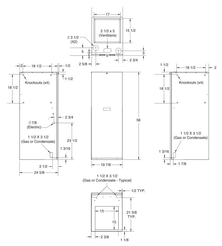
Figure 26. Top Return Cabinets (Without Coil Box)
