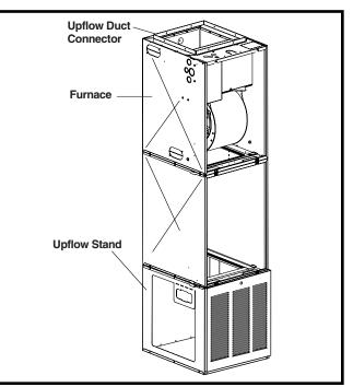
Figure 13. Over-the-Floor Return Air System with Upflow Stand
