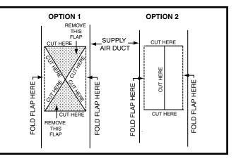
Figure 7. Narrow Air Duct Openings
