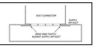
Figure 6. Duct Connector Tabs
