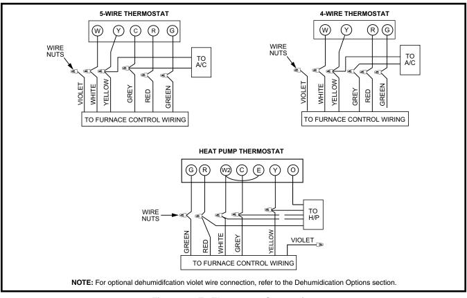
Figure 20. E7 Thermostat Connection
