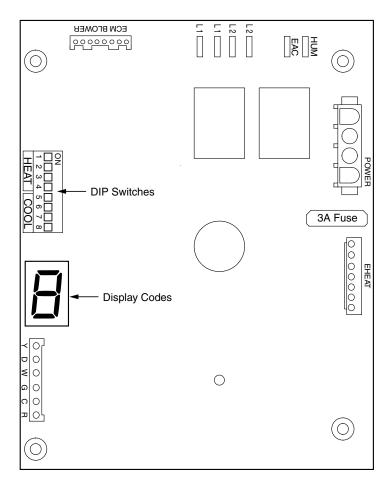
Figure 21. E7 Motor Control Board
