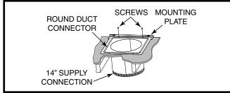
Figure 9. Round Duct Connector Installed
