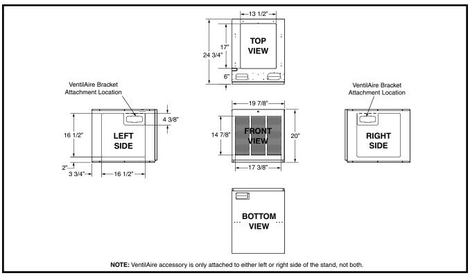
Figure 19. E7 Furnace Upflow Stand Dimensions
