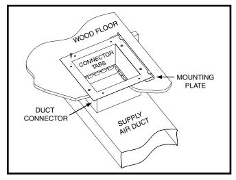
Figure 5. Standard Duct Connector Installed
