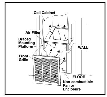
Figure 12. Over-the-Floor Return Air System
