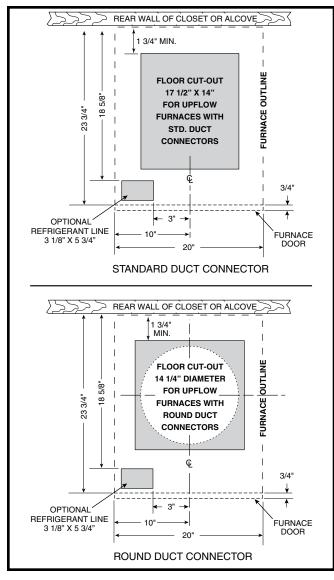
Figure 2. Cut-Out Dimensions for Upflow Furnaces
